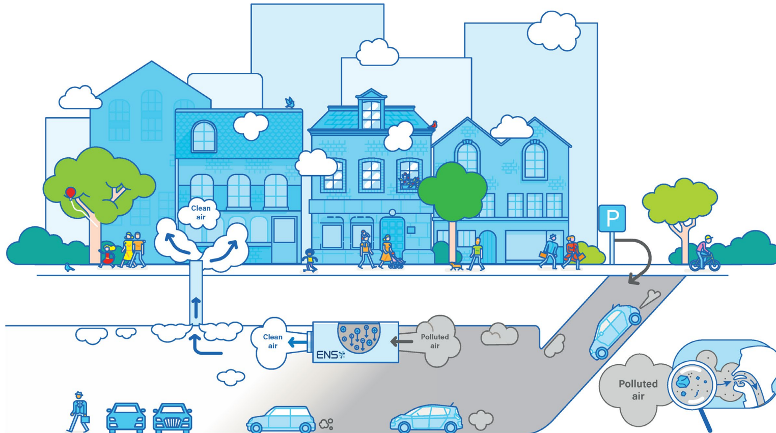
Figure 1 — The principle of the Lungs of the City as applied in an underground parking garage.
