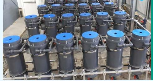
24 ECOTHOR-16R Reactors configured to operate in electrocoagulation mode with ANO2M (Mg alloy) anodes and with Allen-Bradley PLC (customer spec)
